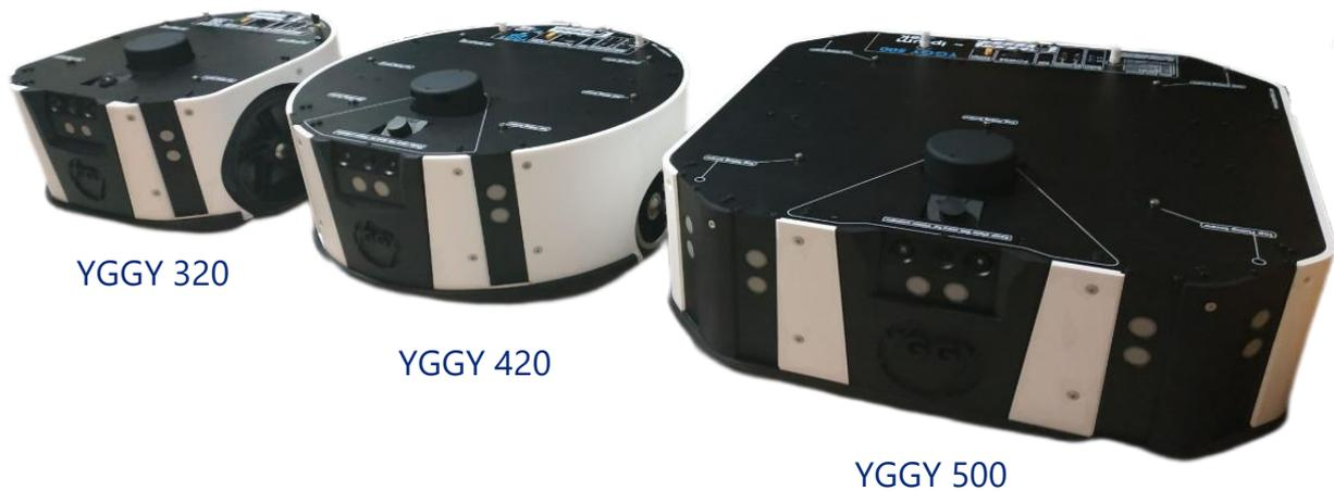
The 3 bases named YGGY 320, YGGY 420 and YGGY 500 get the same functionalities: Localization, navigation, obstacles avoidance and automatic return to their charging station. They differ only by the size, the power, the payload accepted and the battery capacity.
